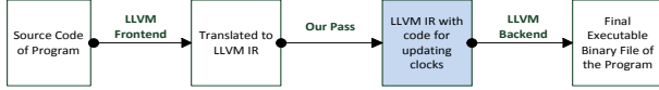
Figure 3. Our tool modifies the LLVM IR code by inserting code for updating logical clocks, used for deterministic multithreading
