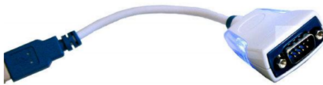
Figure 4.13: FTDI US232R, USB to serial converter .[45].
