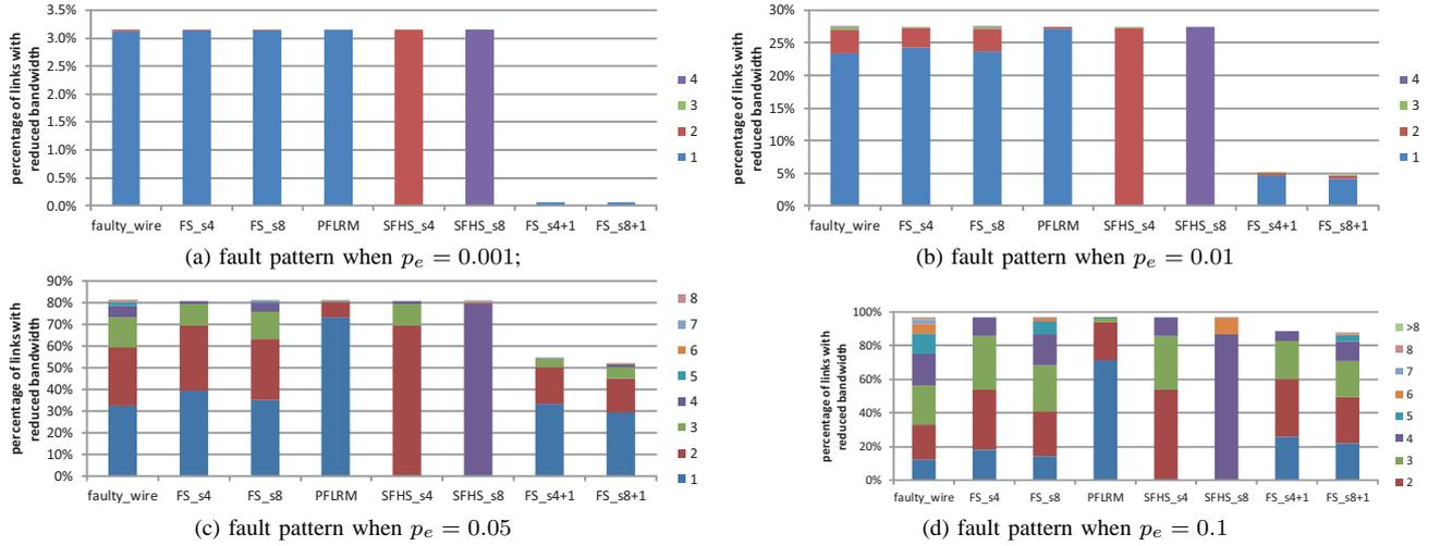
Fig. 8. Fault link Patterns at different wire fault rate. In the FS\_s4+1 and FS\_s8+1 cases, one redundant link section is provided, and links with only 1 broken link section are not counted in as they still can transmit one integral flit per cycle.
