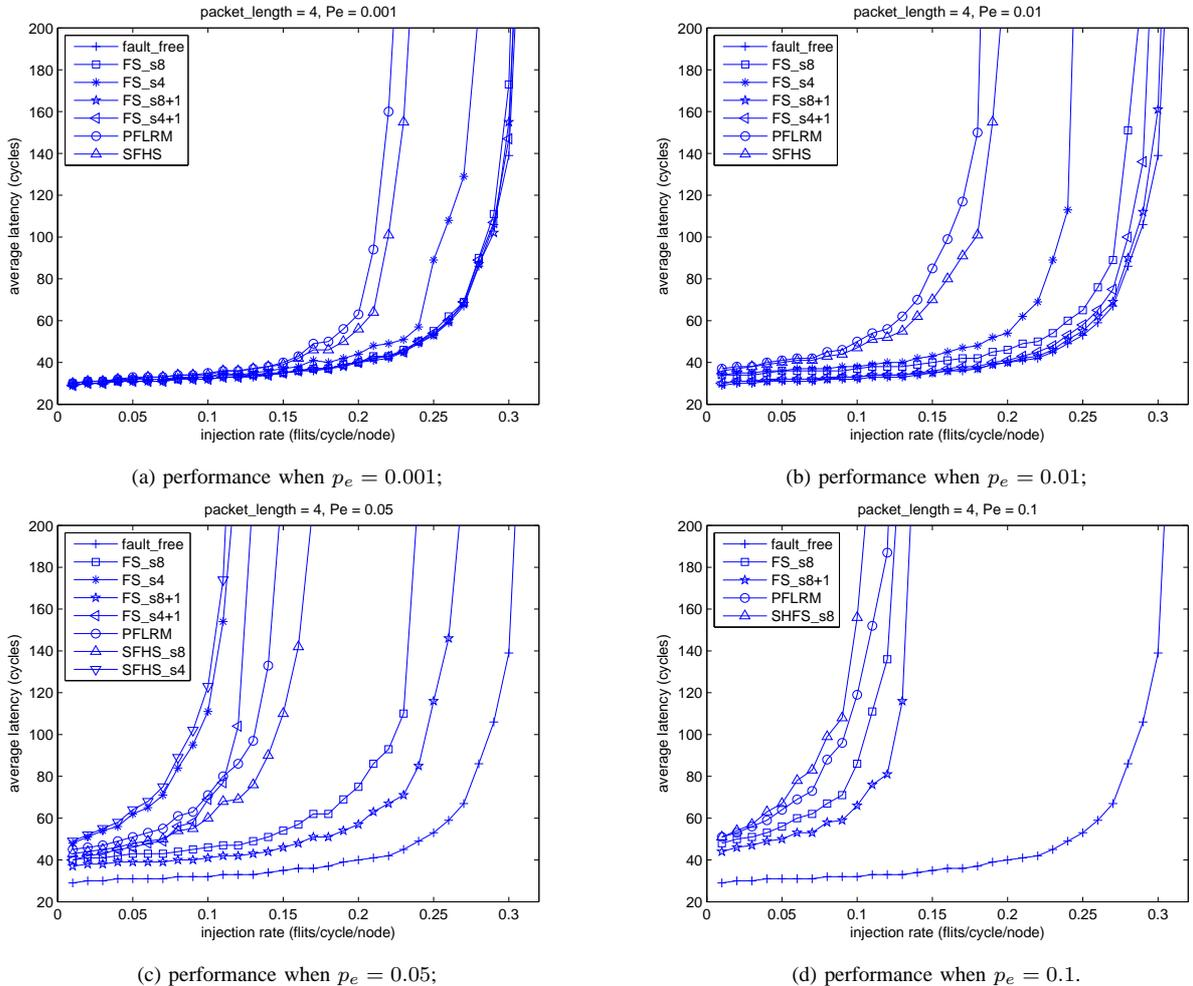
Fig. 9. NoC Performance at different wire fault rate.
