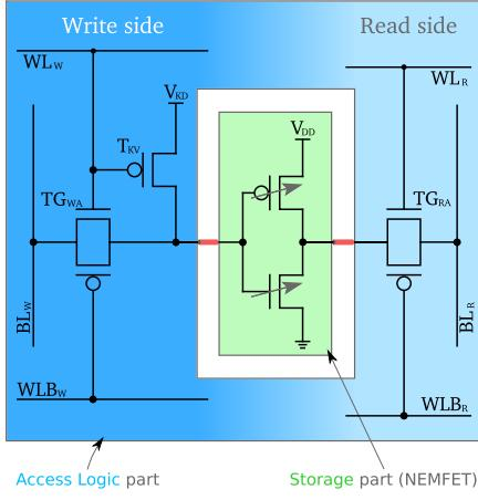
Fig. 3. Hybrid NEMFET-CMOS Memory Cell.
