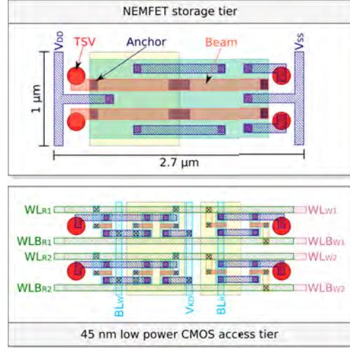
Fig. 4. Two Adjacent Hybrid NEMFET-CMOS Memory Cells Layout.
