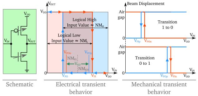
Fig. 2. NEMFET's Inverter Schematic and Transient Behavior.
