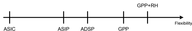
Fig. 1. Positioning of different computer architectures in terms of flexibility. GPP + RH represents a reconfigurable architecture composed by a GPP and a Reconfigurable Hardware (RH).
