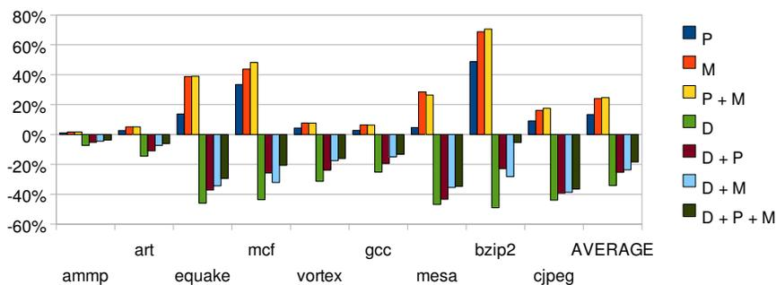
**Figure 5.15:** IPC increase of different precomputation (P), memoization (M), and duplication (D) schemes over the original execution on a system with 2 integer ALUs. Average for different table configurations.
