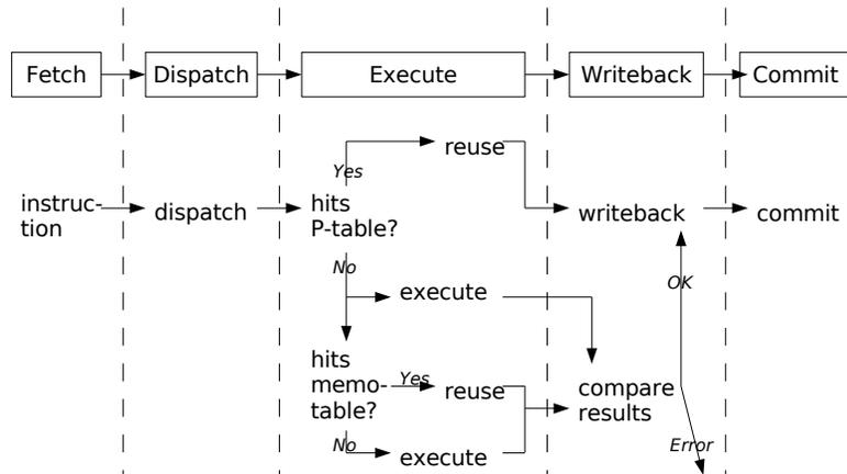
**Figure 5.10:** Instruction duplication with precomputation and memoization (D+P+M). Memo-table update at Writeback (as in Figure 5.9) is skipped.
