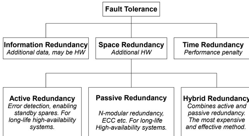
**Figure 2.2:** Protective Redundancy Types.
