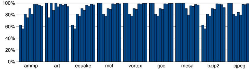
**Figure 5.6:** Precomputation table utilization (% of the whole table). P-table configurations (# sets, associativity) for every benchmark, from left to right: (2,4), (2,8), (4,4), (4,8), (8,4), (8,8), (64,4), (64,8), (128,4), and (128,8).
