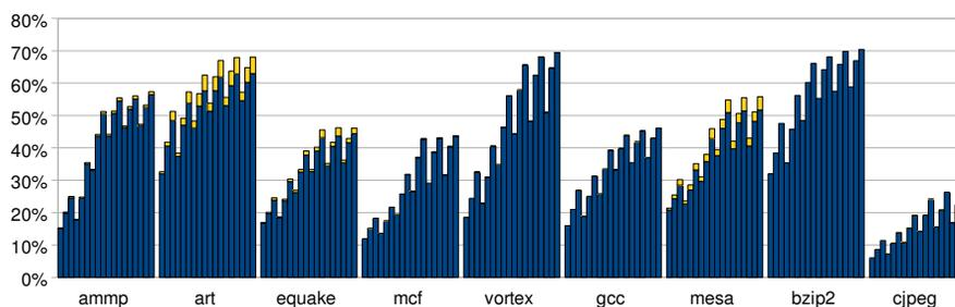
**Figure 5.12:** Memoization hit rates for different table configurations. Upper parts of the bars represent the fraction of reused multi-cycle instructions, lower parts the fraction of reused single-cycle instructions.
