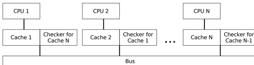
**Figure 6.1:** Proposed system structure.
