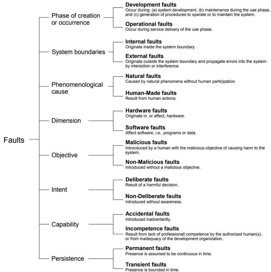
**Figure 2.1:** Faults classification according to Avizienis [1].
