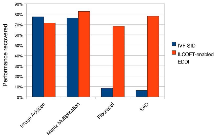
**Figure 4.6:** Comparison of performance penalty reduction achieved by IVF-SID over instruction duplication and by ILCOFT-enabled EDDI over EDDI.
