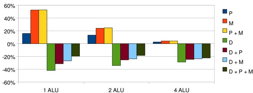
**Figure 5.17:** IPC increase of different schemes with different number of integer ALUs. Average for different table configurations and benchmarks.
