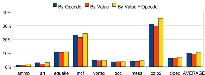
**Figure 5.7:** Performance comparison of three P-table indexing strategies: by opcode, by XORed instruction operand values, and by XORed instruction operands and opcode. Average IPC increase (for the table configurations as in Figure 5.6) over execution without precomputation.
