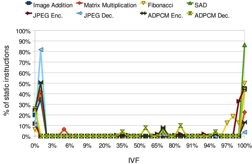
Figure 4.2: Histogram of IVF values for different applications and kernels.
