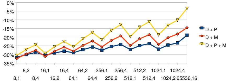
**Figure 5.18:** IPC increase for different table configurations. Average for systems with 1, 2 and 4 integer ALUS.
