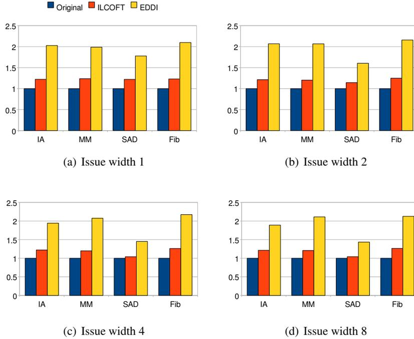
**Figure 3.5:** Energy consumption increase of EDDI and ILCOFT-enabled EDDI over non-redundant kernels, for varying issue widths.
