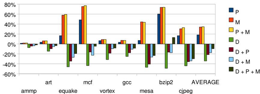
**Figure 5.16:** IPC increase of different precomputation (P), memoization (M), and duplication (D) schemes over the original execution on a system with 2 integer ALUs. P- and memo-tables have 512 sets and the associativity is 4.
