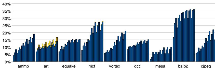
**Figure 5.11:** Precomputation hit rates for different table configurations. Upper parts of the bars represent the fraction of reused multi-cycle instructions, lower parts the fraction of reused single-cycle instructions.
