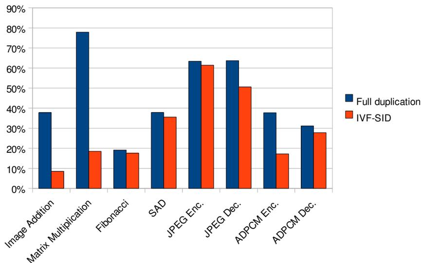
**Figure 4.4:** Performance penalty of instruction duplication and IVF-SID compared to redundancy-free execution. System with 4 integer ALUs, and a fetch/decode/issue width of 4.
