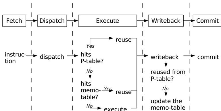
**Figure 5.9:** Instruction precomputation with memoization (P+M).
