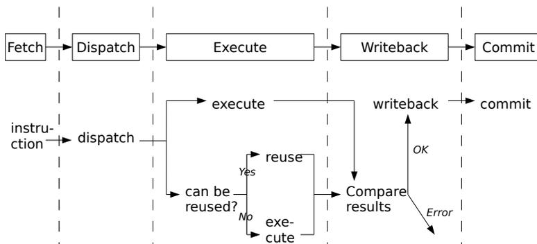
**Figure 5.8:** Instruction duplication with memoization (D+M).
