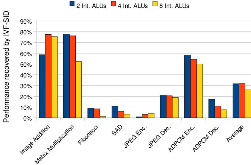
**Figure 4.5:** Performance penalty reduction achieved by IVF-SID over instruction duplication on different processor configurations. Fetch/decode/issue width matches the number of integer ALUs.
