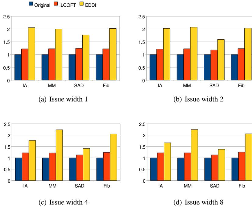
**Figure 3.3:** Slowdown of EDDI and ILCOFT-enabled EDDI versions over the non-redundant version, for varying issue widths.
