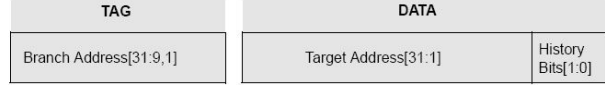
Fig. 2. Illustration of a BTB entry in the case of a bimodal predictor [20].
