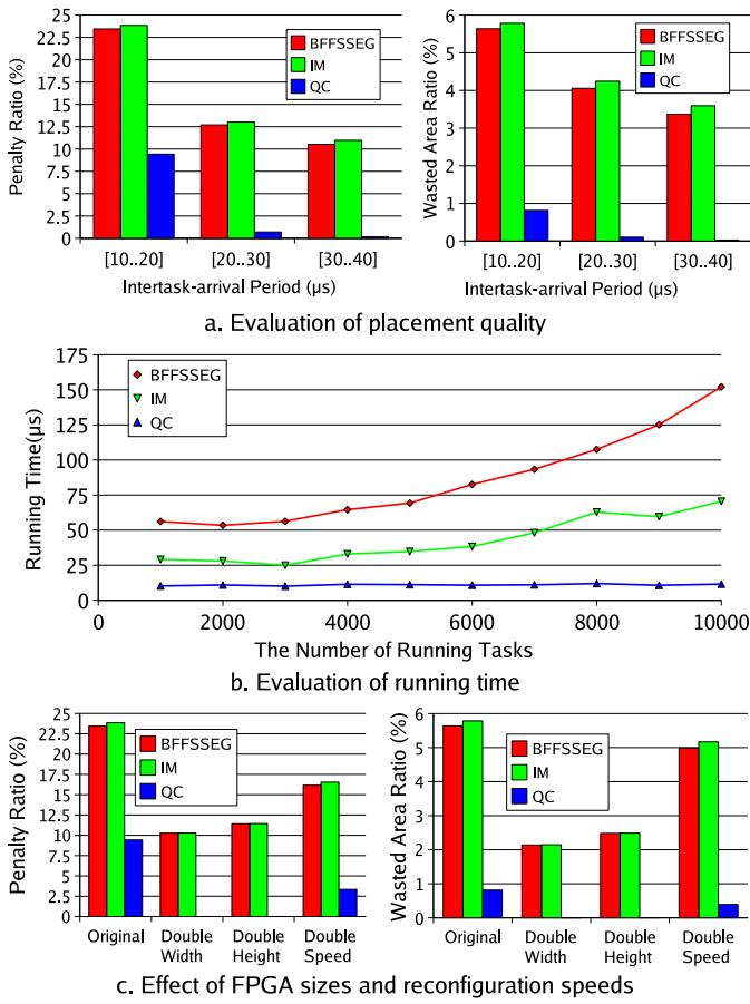
Fig. 4. Evaluation with real hardware tasks
