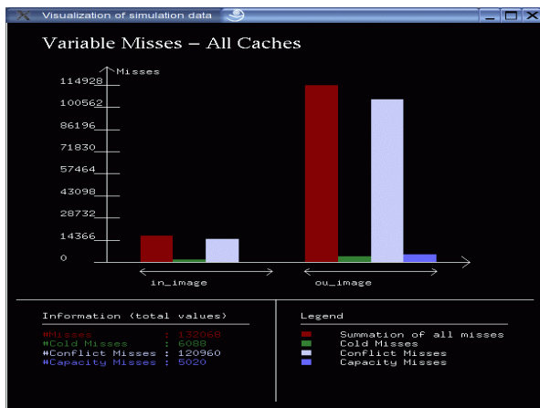
Figure 3. Variable Miss Overview of the 2D DWT implementation.
