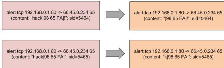
Figure 3.10: Example of extracting a unique part for two rules that have the same header part and their contents differ in just one token. Length was selected to 4 bytes.
