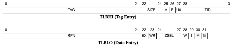
Figure 2.13: Contents of a TLB entry [7].
