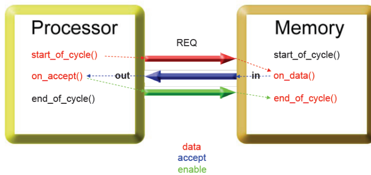
Figure 3.3: Communication protocol between the modules of CellSim, taken from [3]
