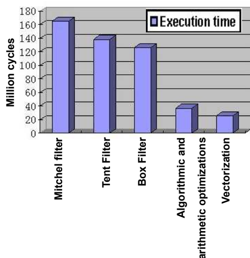
Figure 16: Execution time of the parallax algorithm on a single Trimedia processor.
